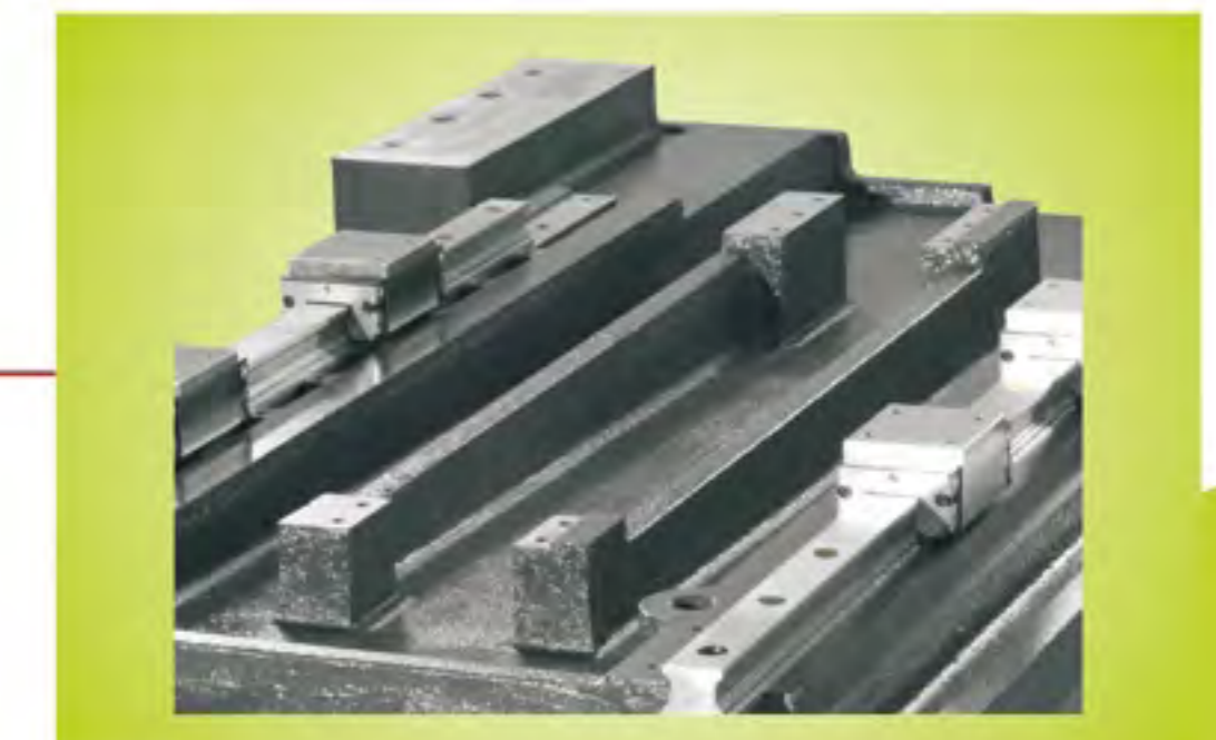
The bearing and the motor seat in Y axis are connected in one piece to have better performance during high speed movement
